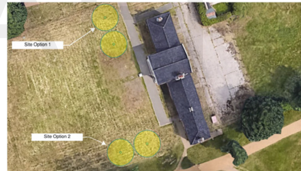
Potential GSHP borehole array locations
